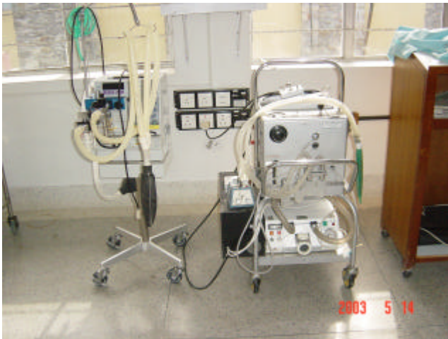
Photo 9: Equipment on rollers in the operation theatre and other places is vulnerable as it may roll and impact with other objects.
