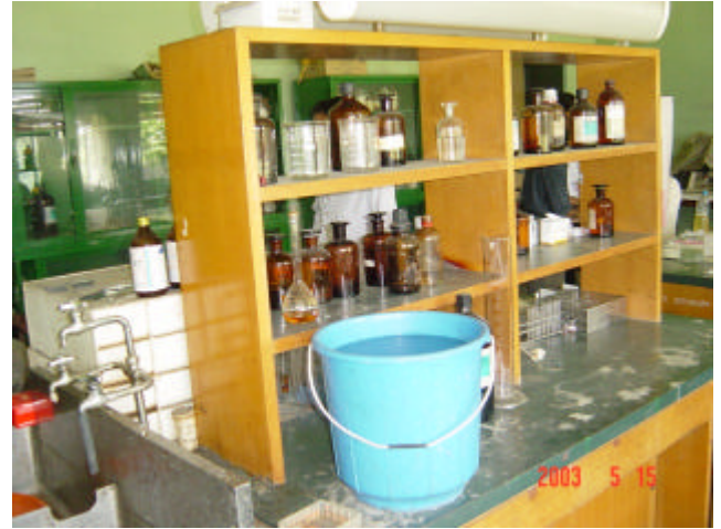
Photo 14: Racks containing chemicals in laboratories should be anchored; chemical bottles should be strapped or relocated to improve safety conditions.
